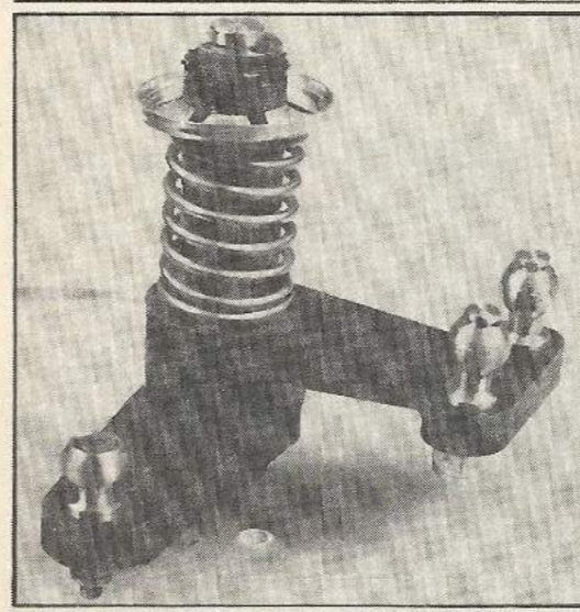
▲ Radio plate installed with wire outriggers to carry receiver and battery. Servo recess is to take the smaller Futaba and has been nicked to let the lead through.
